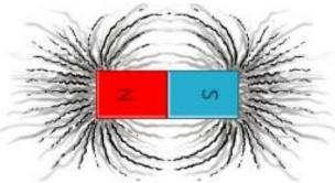
If we put iron filings around the magnet then the magnetic field can clearly be seen.
