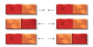
Each side of a magnet is different. Magnets have both North and South poles. Similar poles repel each other, such as North with North, whilst opposite poles attract, such as North and South.
